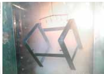
STAGE 3: PRE-RINSE Rinses off carry-over detergents.
