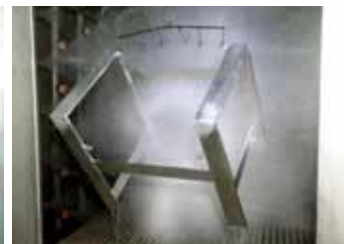
STAGE 4: RINSE Final rinse prior to chemical application.
