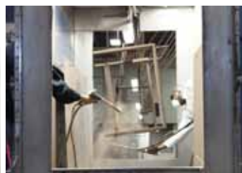
STAGE 7: PAINT APPLICATION Electrostatic equipment is used to consistently coat all areas of the frame.
