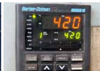
STAGE 8: PAINT CURE Powder-coat cures at an oven temp of 420 degrees for 22 minutes.
